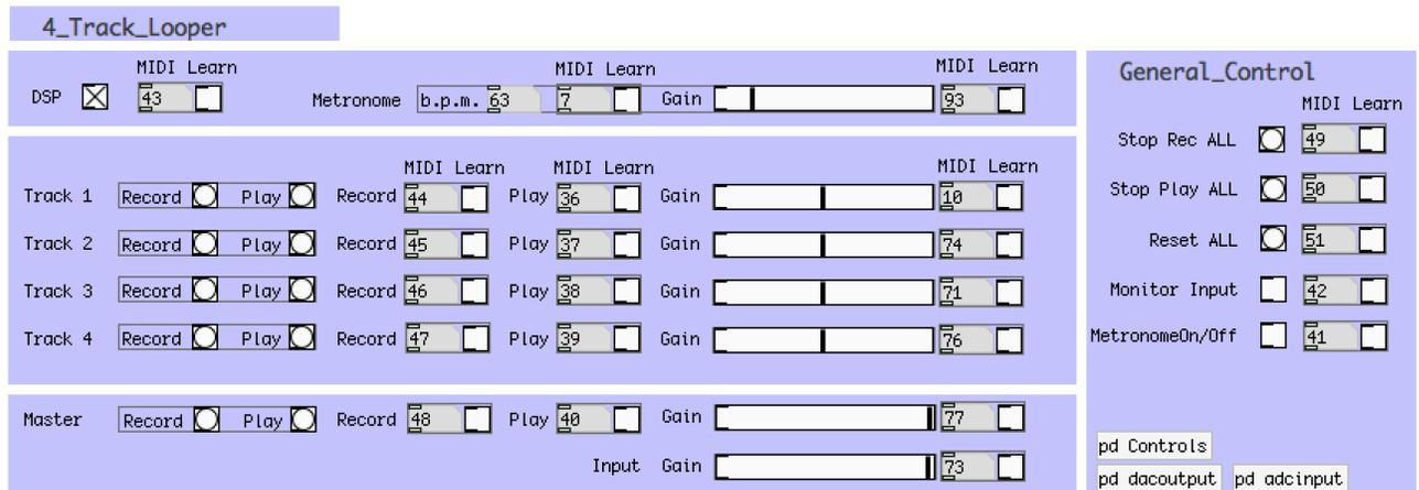
This patch records and loops up to 4 individual tracks. The four different tracks are then sent to a master track than can record and play the final mix. The audio is stored in 5 (4 tracks and master) wav files in the folder where the path is located.
